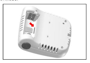
Replace the protection strip then the battery, ensuring that the battery is placed in the correct direction of polarity.
